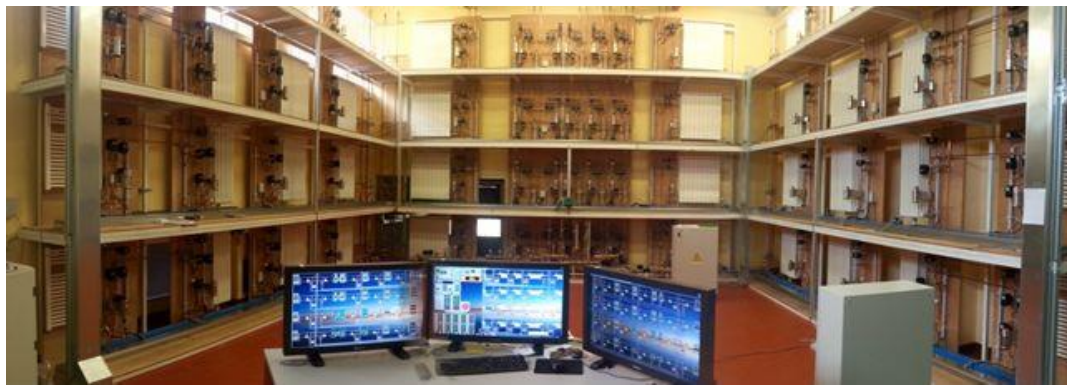
182 Figure 3 - Heat accounting experimental mockup at INRIM
