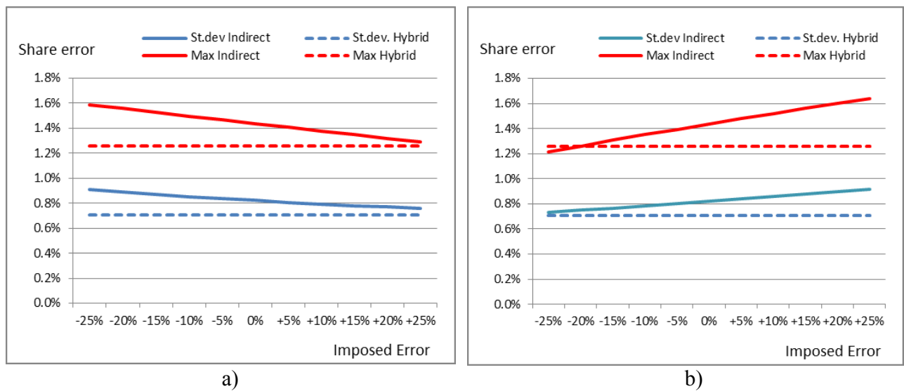
388 Figure 8 – Sensitivity analysis of the K coefficient estimation of radiators: a) error in only one raising 389 main (1N), b) error in two raising mains (1N e 3S)
