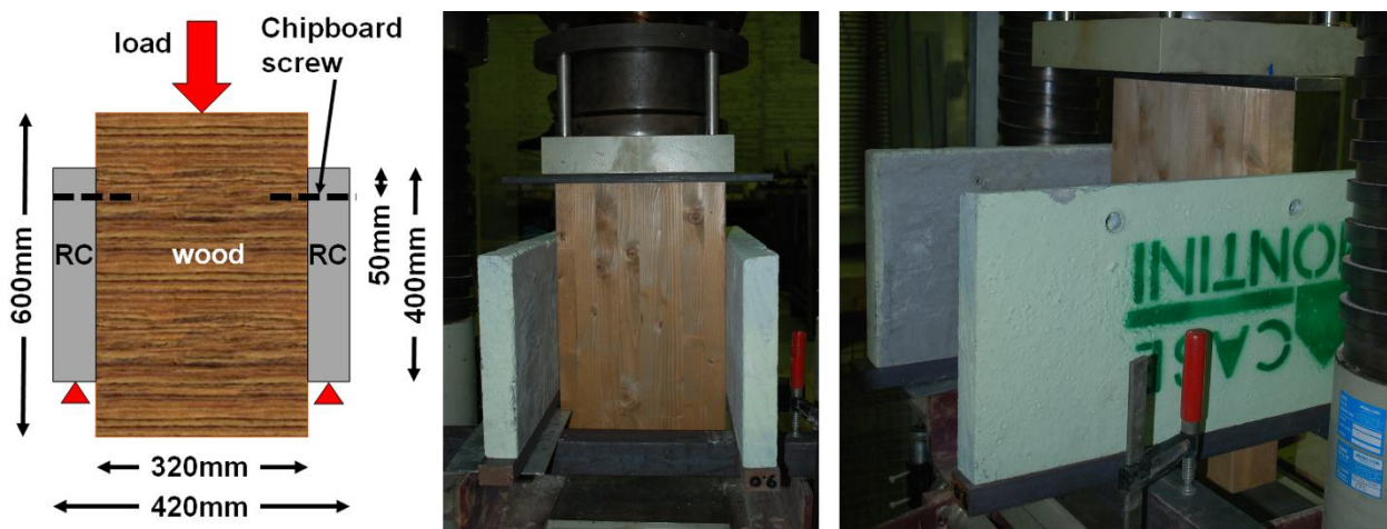
Figure 5. RC-wood specimens, scheme and setup.
