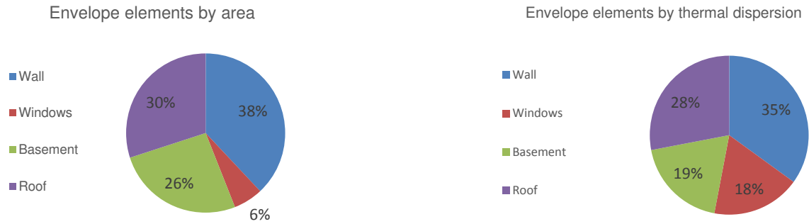
Figure 10 – percentage distribution of the envelope elements by area and by thermal dispersion
