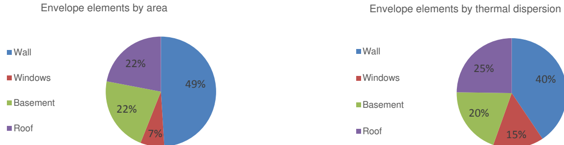
Figure 4 – Distribution of the envelope elements [%] by area and by thermal dispersion
